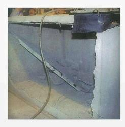
FORTA® technicians performed a vacuum test on a steel-reinforced 1,000 gallon single piece tank produced in Clarion, PA. The steel reinforced tank passed both ASTM and NPCA minimum standards, and showed catastrophic long wall collapse at 9-10 in. of mercury.
